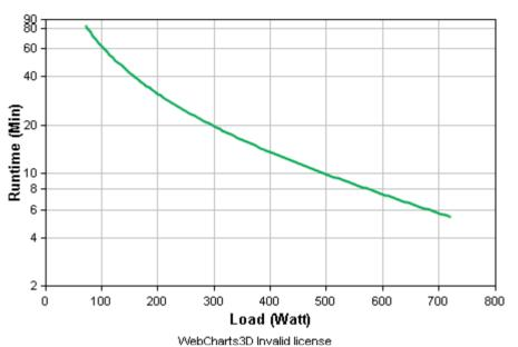
Curve fit to measured runtime data. All measurements taken with new, fully charged batteries, at typical environmental conditions, with no electrical input and balanced resistive load (PF = 1.0) output.
