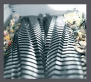
Cutting unit stage 2: downstream shredder The HSM DuoShredder 5540.2 is a two-stage shredder system for fully automatic document disposal. Depending on the paper quality, loading and downstream systems, it can achieve a throughput of up to 350 kg per hour. In combination with an HSM baling press, you can expand the HSM DuoShredder 5540.2 into a complete disposal system. We recommend the following baling press models: HSM KP 100.1 and HSM KP 88.1.
